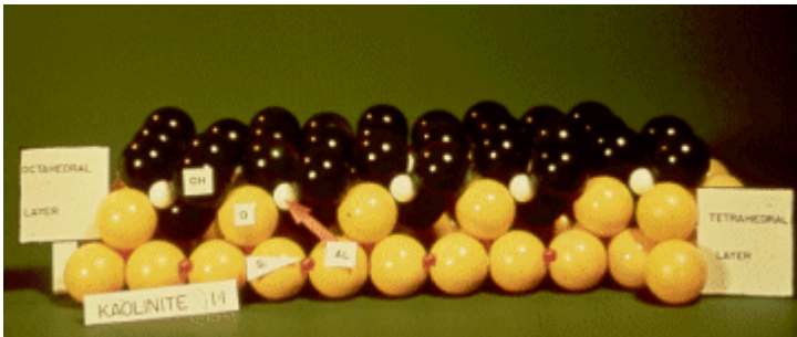
Figure 3.8 Kaolinite clays are composed of one layer of silica and one layer of alumina.
